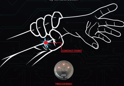
CONTACT (sur individu): Grab the assailant, avoiding the areas considered dangerous (eyes/jugular/testicles). Upon contact of the glove with the assailant, the contact button located in the middle of the palm of the hand will trigger the electrical impulse (Triggering).
