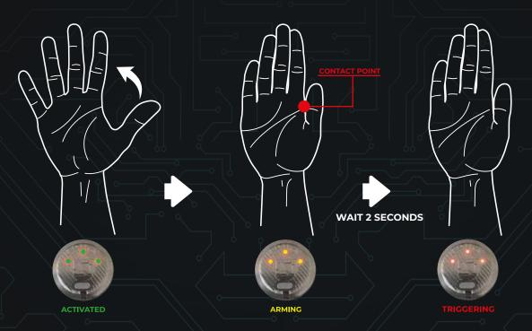
DISSUASION (remotely): Move your thumb towards your index finger to activate arming. After 2 seconds, the electrical impulse will be triggered. (Triggering).
